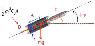
Figure 2: Rocket model in 2D during ascent phase
